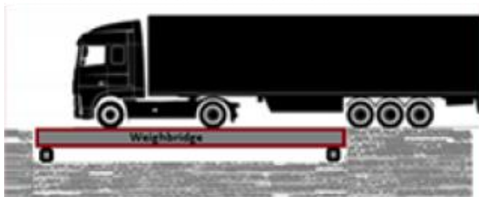
Truck and trailer coupled, with only the truck on the weighbridge
