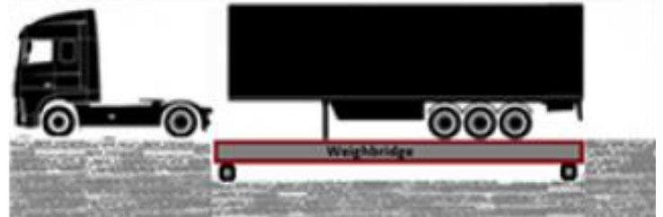
✓ Truck not on the weighbridge, with the uncoupled trailer on the weighbridge
