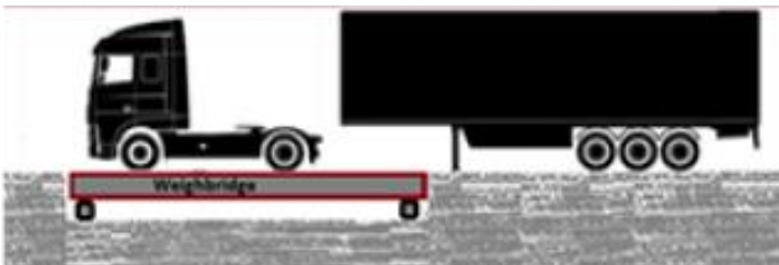
✓ Truck on a weighbridge, with the uncoupled trailer not on the weighbridge
