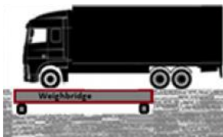
Truck with only its front axle on the weighbridge
